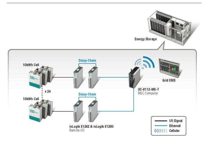
An energy storage system provider in the US was commissioned to build a 40MWh energy storage system for a key customer in the solar power industry. It was quickly determined that the customer could benefit from using an IIoT setup, which involves connecting various
