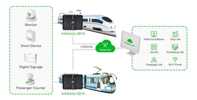
Devices on board, including monitors, smart terminals, digital signage, etc. are connected to the VG810 through extensive interfaces. Data from within the vehicles are collected
